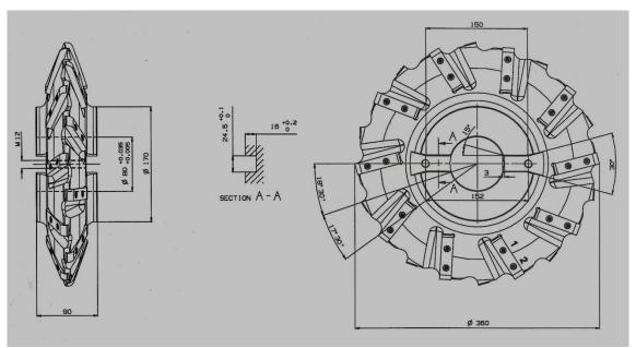
Figure N°8- Insert milling cutter for finishing operation
