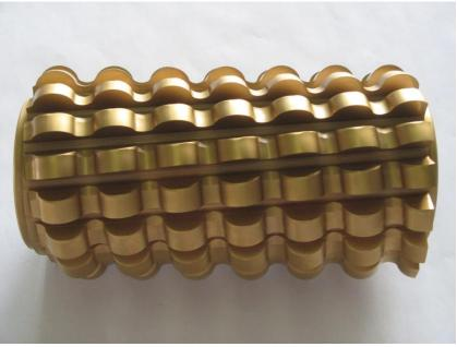
Figure N°6 – Hob for roller chain sprocket
