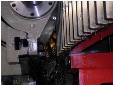
Figure N°1- Hobbing of a big gear
