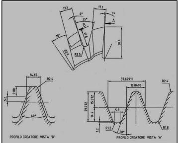
Figure N°4- Different shape of teeth in a hob module 12 mm
